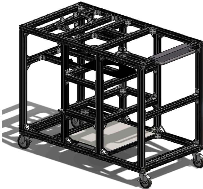
Figure 18. Finalized design featuring more extrusions to allow for better support of the pulley system, as well as a bottom panel to hold various cooling system components.
